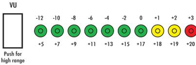
VU METER - An LED meter that functions in two ranges. The ranges are from -12 to +3 and +5 to +20db. You can select the range with the pushbutton to the left of the meter.
